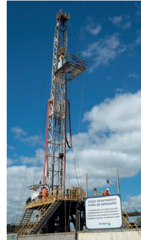
Probe used to check integrity in Braskem disabled rock salt exploration well
